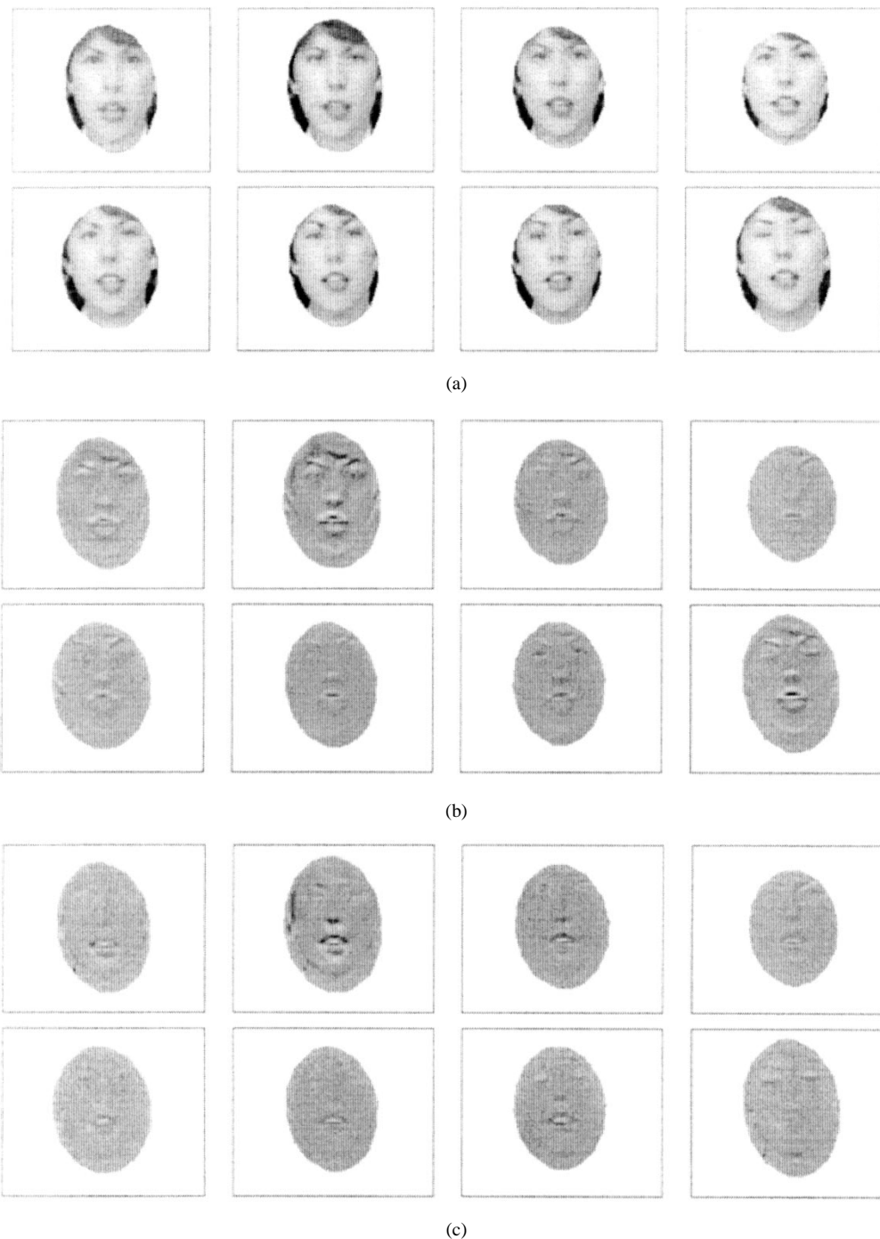
Fig. 13. Motion estimation results for the “Claire” sequence. (a) Motion compensated frames 1–8. The original can be seen in Fig. 4. (b) Difference between original consequent frames. (c) Difference between original and motion compensated frames.
