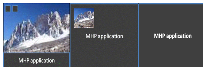
Fig. 10: Card Display Modalities: Stripe, Full Screen with TV Picture, and Full Screen Instance of a Multimedia Page.
