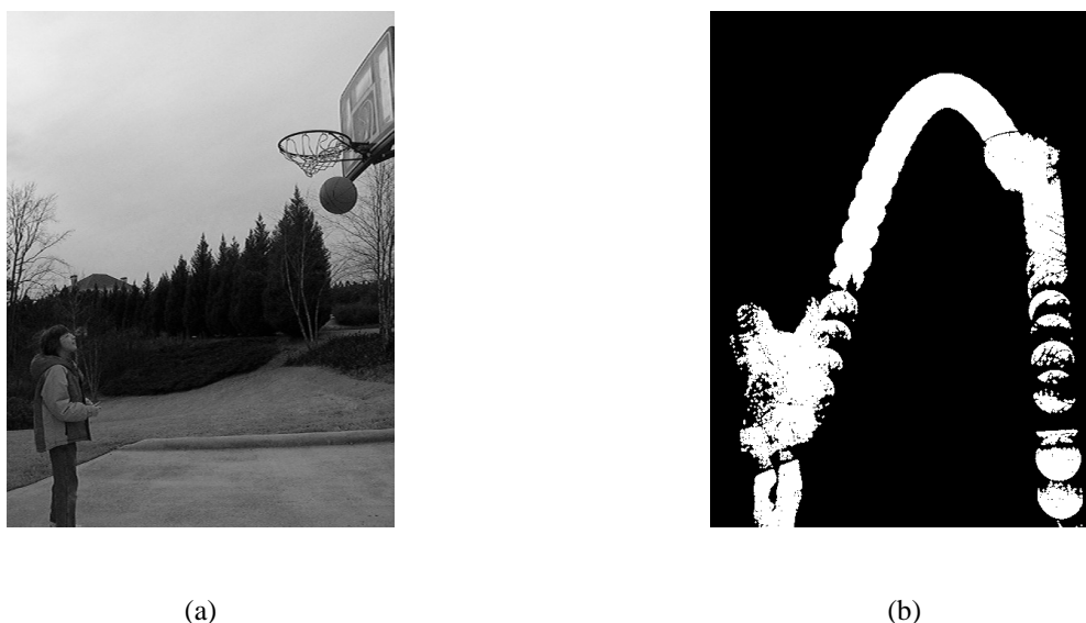
Figure 2. (a) Video frame of kid playing basketball. (b) Active pixels during the shot.
